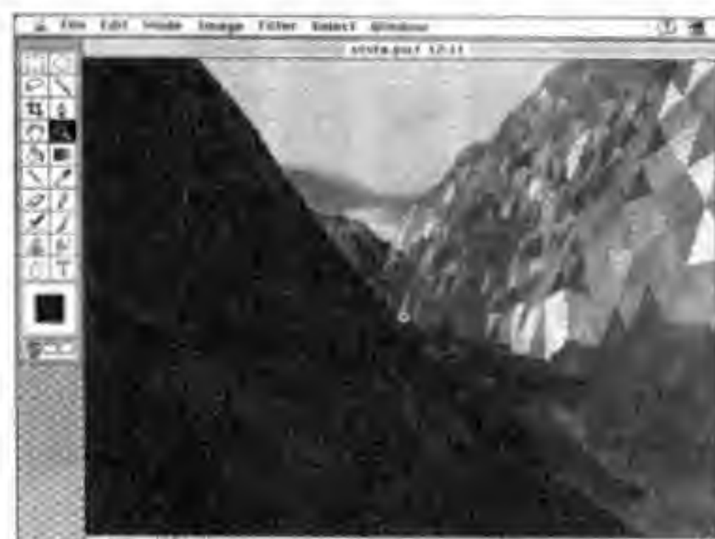
The Mac image processing program Photoshop running in 256-colour mode (honest), with a 24-bit file generated by Vista Pro 3 on the Amiga.
